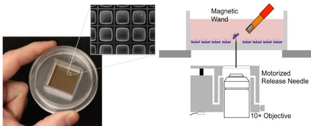
**Figure 2:** The CytoSort™ Array. Raft features are 200X200 microns, with about 10,000 rafts per array. The release needle is positioned on a collar fitted to the imaging objective. The magnetic capture wand is applied by hand to capture and transfer the CellRaft.
