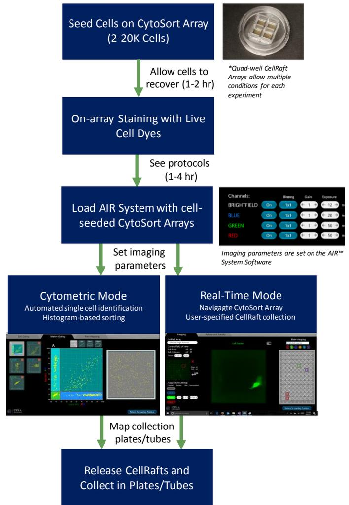
**Figure 3:** The AIR™ System workflow allows customized imaging settings followed by either “real-time” selection of single cells for isolation, or “cytometric” sorting using histogram-based gating of fluorescent signals prior to isolation of single cells.
