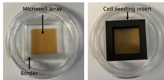
**Figure 1.** CytoSort™ Array shown with and without cell seeding insert. Black prototype of insert is shown for visualization (actual insert is clear polystyrene).
