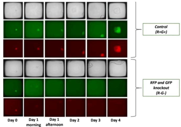
**Figure 3:** Single cell suspensions were seeded on the CytoSort Array and imaged on the AIR System each day for 5 days (Day 0 = day of transfection). Each scan required 15 minutes, and arrays were placed back into a standard laboratory incubator between scans. By imaging, colonies were monitored for inclusion of extraneous cells to ensure clonality. Presence of cells in each microwell was confirmed with brightfield imaging.
