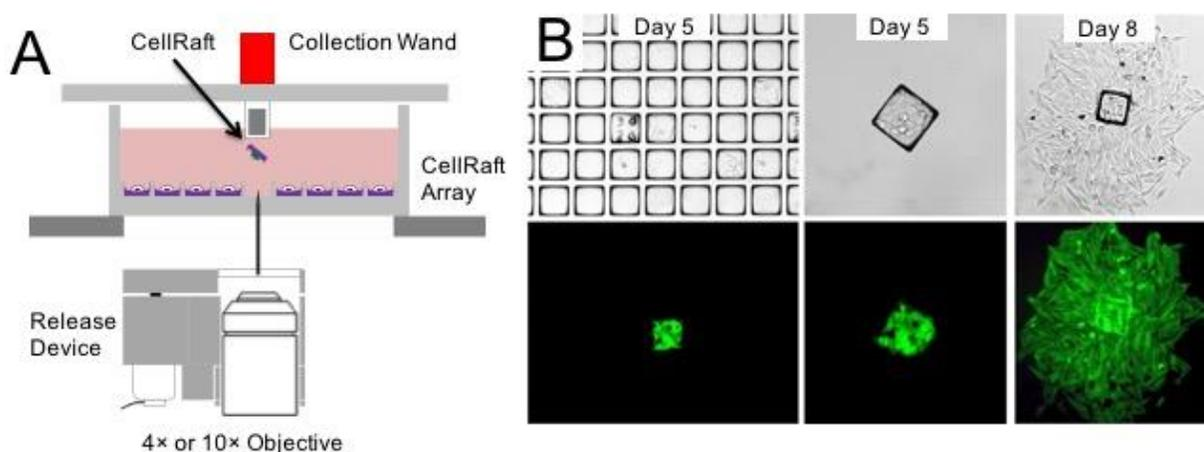
**Figure 1.** CellRaft® System for Inverted Microscopes. (A) Schematic of the working principle of the CellRaft® System. (B) Example of sorting GFP-H1299 cells out of a mixture of cells. A mixture of GFP-H1299 cells and wild-type H1299 cells were plated as single cells on the CytoSort™ Array. At day 5, a clonal fluorescent colony was identified and released from the CytoSort™ Array. The recovered colony was expanded in a separate Petri dish for an additional 3 days.
