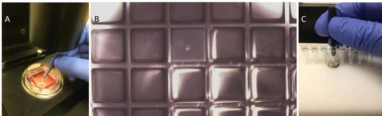
**Figure 7.** CellRaft Collection and Deposit. (A) Magnetic Collection Wand inserted into media to collect a released CellRaft. (B) Wand tip shadow indicating alignment with released CellRaft. (C) CellRaft deposit into a PCR tube using the Magnetic Collection Plate.
