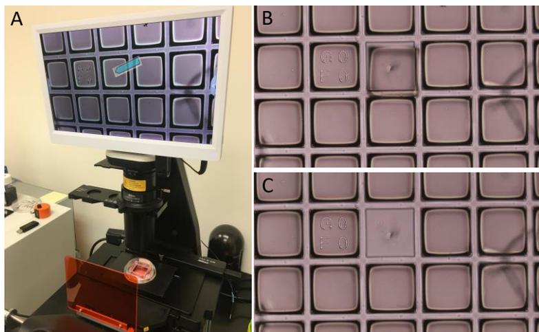
**Figure 6.** CellRaft Release. (A) Alignment of target CellRaft with needle release position. (B) Target CellRaft dislodged from its microwell. (C) CytoSort<sup>™</sup> Array after collection of target CellRaft.
