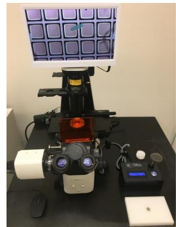
**Figure 4.** Controller and full CellRaft® System setup.
