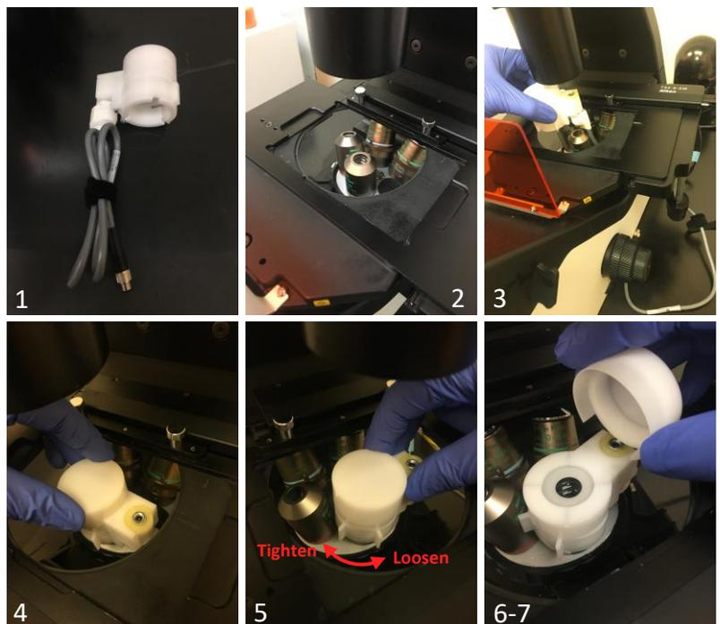
**Figure 2.** Installation of the Motorized Release Device.
