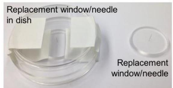
Figure 8. Replacement window and needle assembly.
