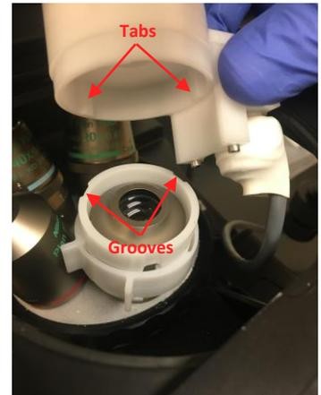
**Figure 3.** Removal of release device with collar fixed to objective.
