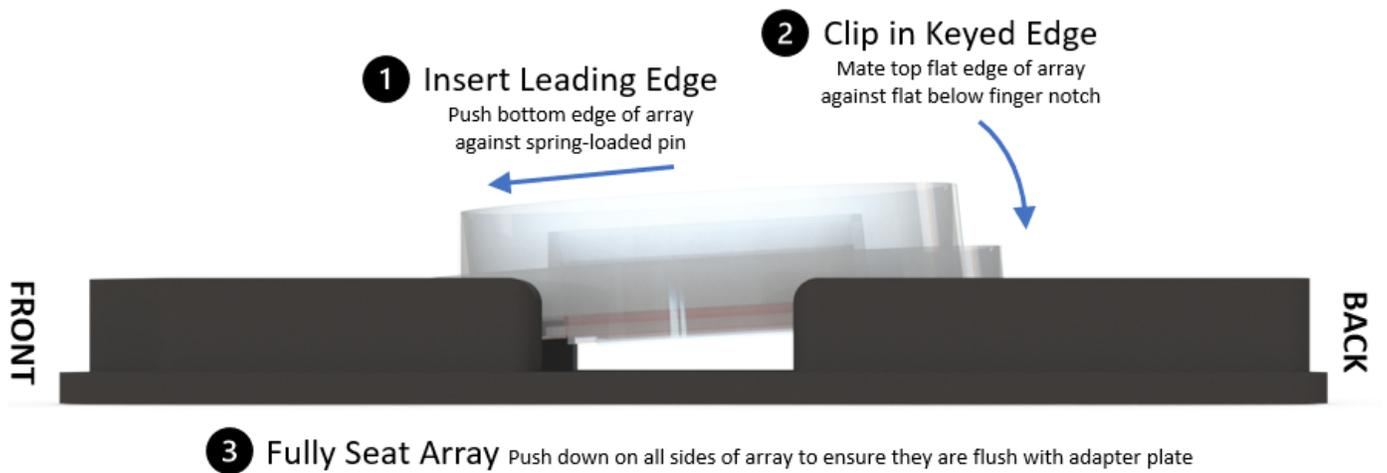
To load a CellRaft Array into the Adapter Plate, it is best to grip the array with your thumb on one side, index finger along the flat next to the Keying Arrow, and remaining fingers on the opposite side. Then:
