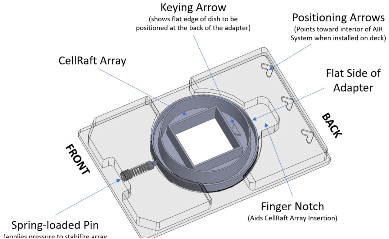
Every 65-mm CellRaft Array contains a flat section along its outer circumference, whose location is indicated by its Keying Arrow (as shown in **Figure 1**). To standardize array orientation between runs on the AIR System, the CellRaft Array Adapter Plate contains a complementary flat below its Finger Notch, so the array can only be inserted into the adapter with the two flats aligned.
